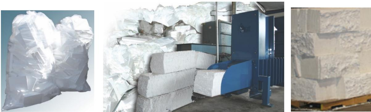
The Bright D30 Densifier is fed by a conveyor that fills a hopper with EPS. The machine then uses cold compaction to densify the foam into blocks at a rate of up to 300 pounds per hour. (The Bright D120 can process even more EPS, up to 1,200 pounds per hour.)
