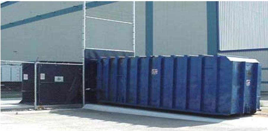
Through-the-Wall/Fence installation, eliminates the need for Security Clearance; the Waste Hauler can switch-out containers from outside the fence area.
