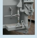
The ratchet latch tightens against the door seal and insures a tight seal.
