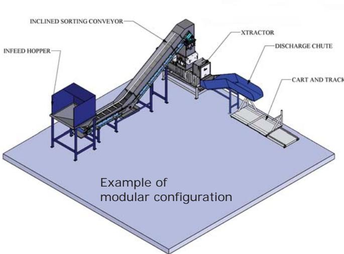
A Xtractor system can be designed with a hydraulic dumper, conveyor or manual loading.
