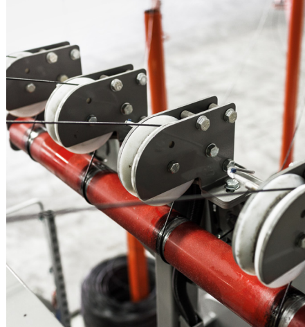
Monitoring of wire breakage and wire end to control the binding wires
