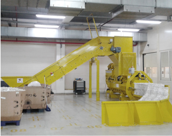
Version with sliding belt conveyor
