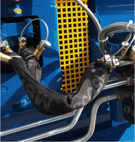
Hydraulic hose with safety trap and burst protection
