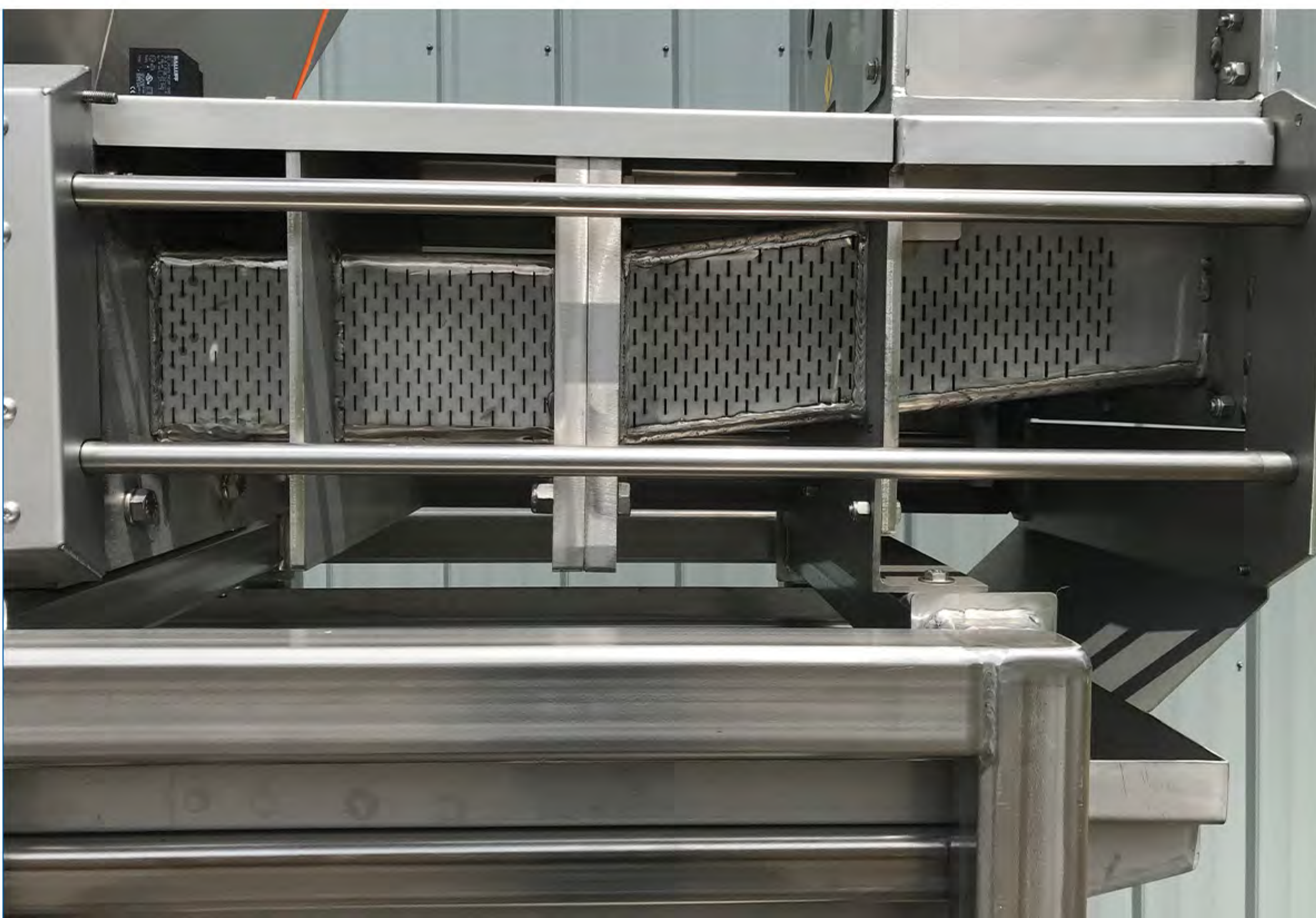
Dewatering Chamber shown
