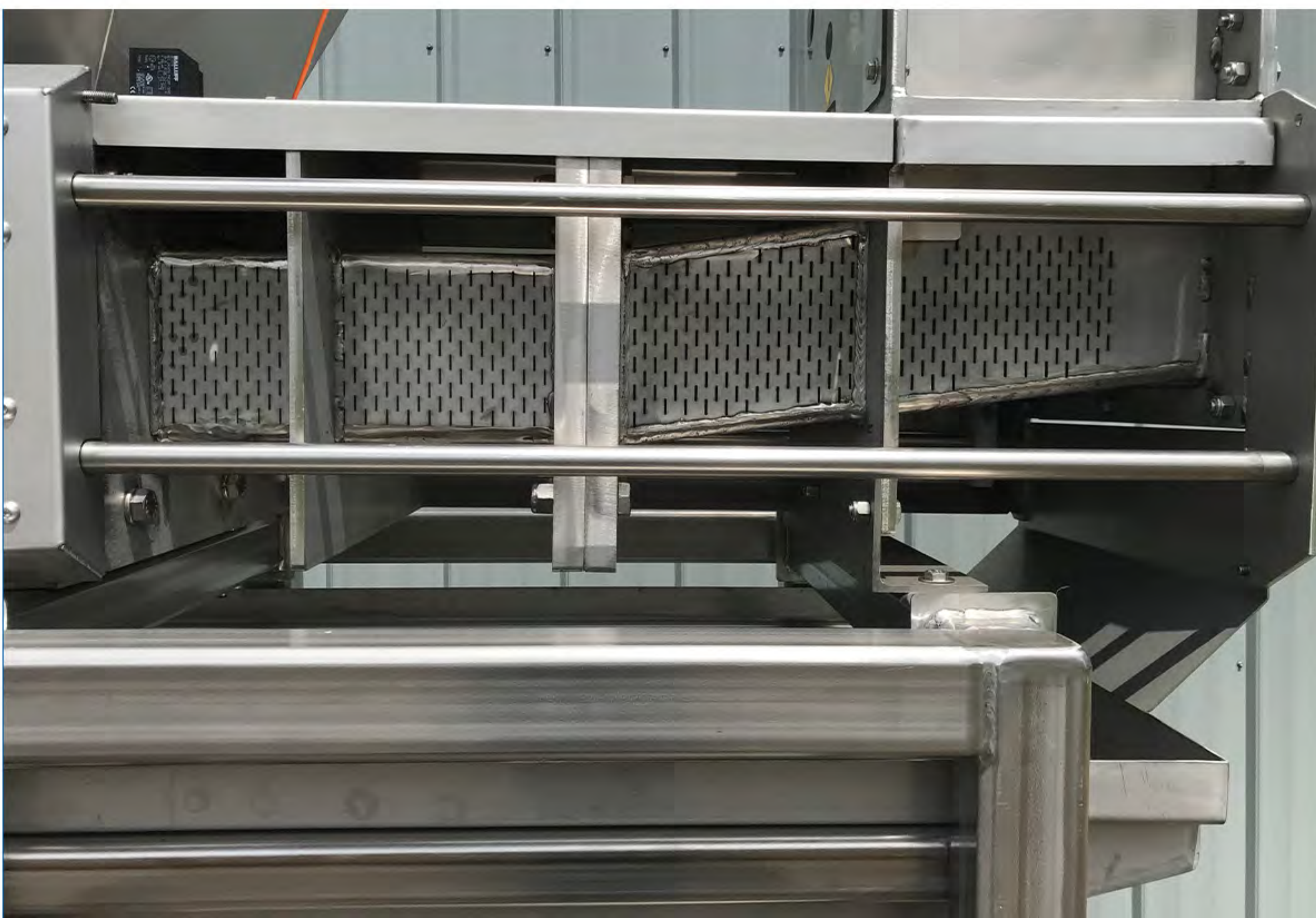
2013X Dewatering Chamber Shown
